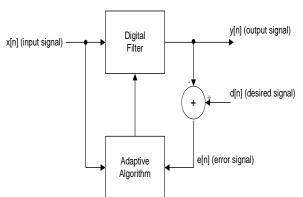
Fig.1. Basic Adaptive filter model [10]
